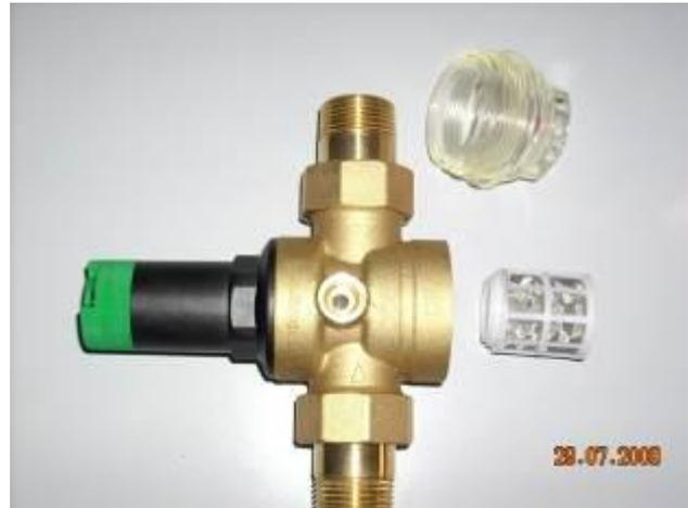
Extract filtering element taking care not to spoil the gasket. Then eliminate all the impurities from the filtering net with compressed air and wash the component with clean water. At the end of the operation, reassemble all the components taking care to the correct placement of the gasket.
