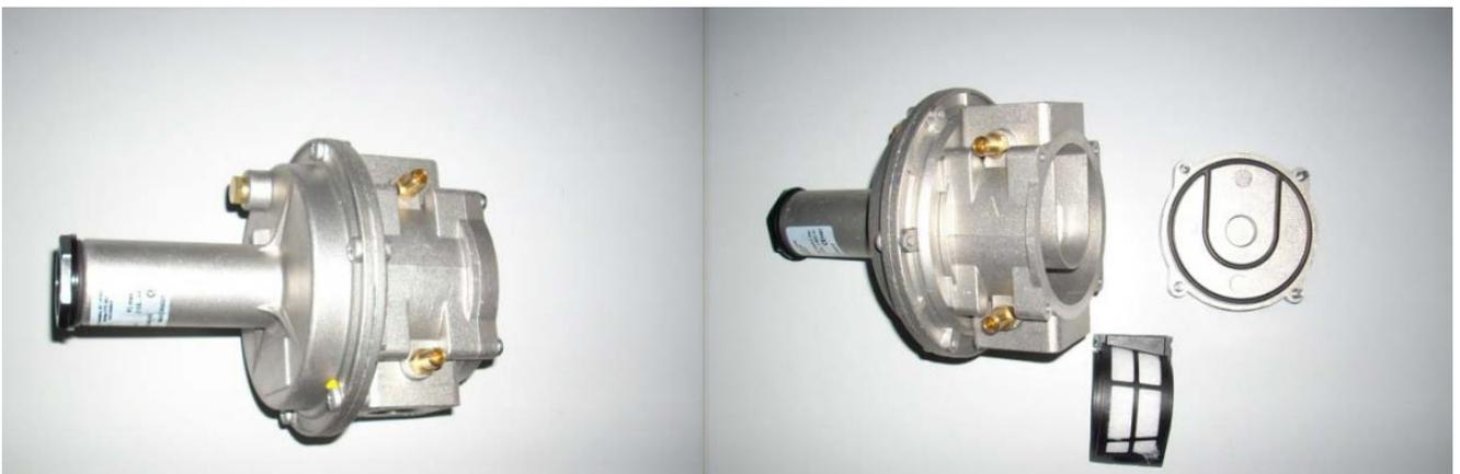
The gas pressure regulators contain a filtering membrane whose task is to capture the impurities coming from the gas net. If this filtering membrane gets dirty or clogged this means that some impurities are present in the gas supply, and these could potentially damage components located on the gas circuit and especially the gas flow transducer.
