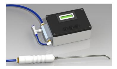
Nasagas SA 2.1 is composed of a main unit and a sniffer, connected to each other by a flexible sheath.
