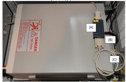
22. Temporarily remove the optocoupler. Be aware that the optocoupler protects the EST unit, therefore it has to be restored (or replaced) before releasing the test bench for ordinary use.
