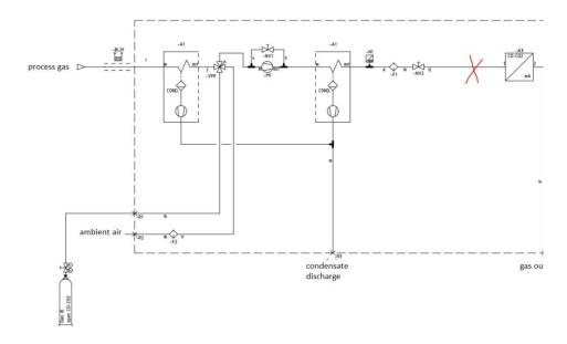
Following the hydraulic diagram, disconnect one by one the pipes of the circuit, and dry them by inflating compressed air. When done, reconnect all the pipes in their original position.
