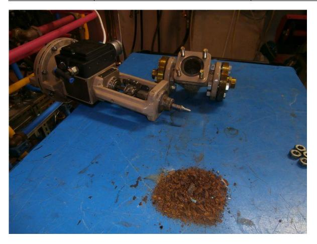
G) Re-assemble the hydraulic body to the valve (screw the 4 bolts) and connect the valve to the test bench (hydraulic, pneumatic and electric connections). When done turn-on the test bench, open air and water supply manual valves and use the cursor bar of the diagnostic program to double check correct operations of the proportional valve, for instance producing a variation of water flow rate.
