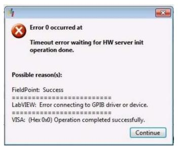
Error 0 might be displayed when switching on the test bench. As a matter of fact the initialization of Microplan hardware server requires some time (some seconds) therefore we introduced a control to make sure that, after a certain time (timeout), fixed by our software engineers, the initialization is concluded.
