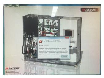
Error 33162 is usually displayed when the communication between the PC of the test bench and the electronic I/O modules is interrupted.
