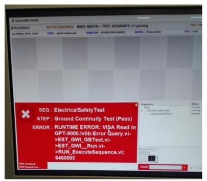
The mentioned problem is very likely to be originated by an unstable/defective communication between the PC of the test bench and the electric safety tests unit.
