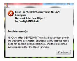
This error indicates a communication issue between the Microplan test bench PC and either CO2WF or FFA Microplan fumes analysers.
