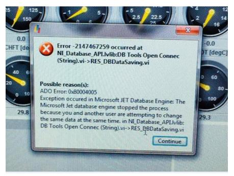
This error might appear with Parseq software and indicates an issue occurred when the test bench was trying to complete the data saving of the tests results.
