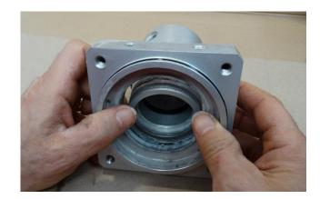
STEP 9: Holding the cylinder in a vise, use two screwdrivers to remove the inner gasket. Lubricate gasket 4 (Teflon grease) and insert it in the cylinder.
