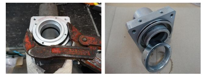
STEP 8: Slide the cylinder out of the plate.
