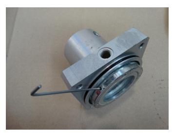
STEP 6: Remove and replace gasket 5. Get it greased (Teflon grease) before it is mounted.
