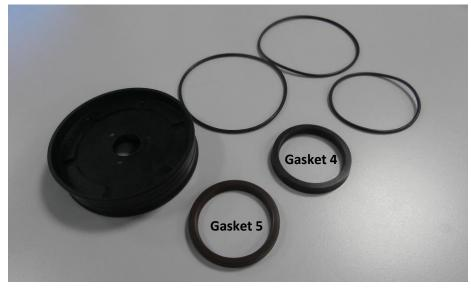
Note: Be aware that the thickness of gaskets 4 and 5 are not identical: Gasket 4 is 7 mm and Gasket 5 is 6,5 mm. Both gaskets should be replaced as follows.
