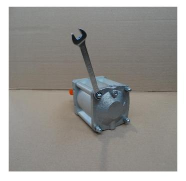
STEP 3: Disassemble the three main units: cover, body, and cylinder.
