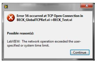
Error at TCP Open Connection, which might appear as Error 42, Error 56 and Error 59, is displayed whenever the communication between the PC of the test bench and the electronic I/O modules is interrupted.
