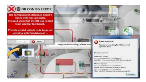
DB config error is displayed under Parseq, Labsoft and R&D flex software environments whenever customers copy a config file from one test bench to another, change the network card of the PC or replace the PC.
