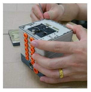
Warning: pay attention to the central gasket positioning and to the lateral gasket to be well positioned, to avoid leakages.
