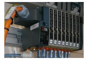
Scope: guide to how to assemble-disassemble a Metalwork Multimach HDM pilots manifold
