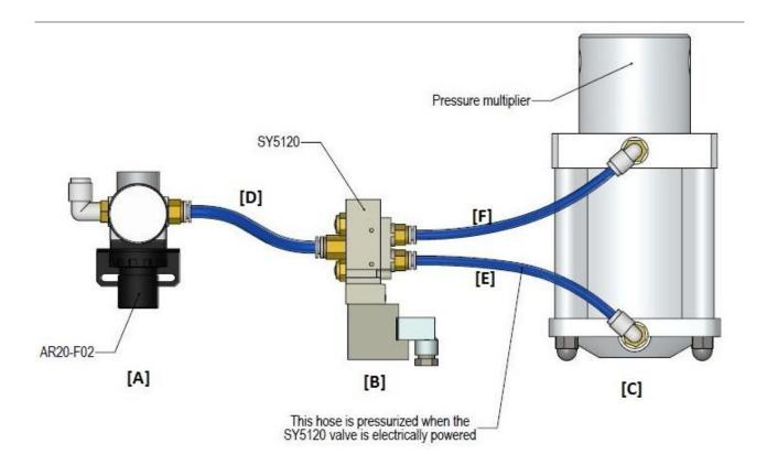
Problem B: water has flown in the pressure multiplier's air pipes [D] [E] [F]
