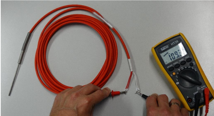
Resistance vs. Temperature - Pt100 (385)
